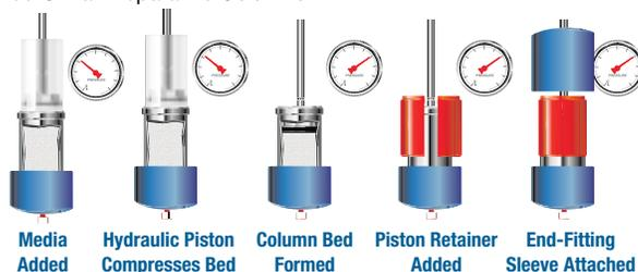
The Axia process uses highly controlled pneumatic mechanical pressure to drive the piston into the column to produce a uniformly packed bed. Once the bed is formed the pressure on the piston and bed is not released, the bed is not disturbed and the piston is locked in place leaving the chiral media under pressure. This packing process won the 2006 R&D 100 Award for its innovation.
