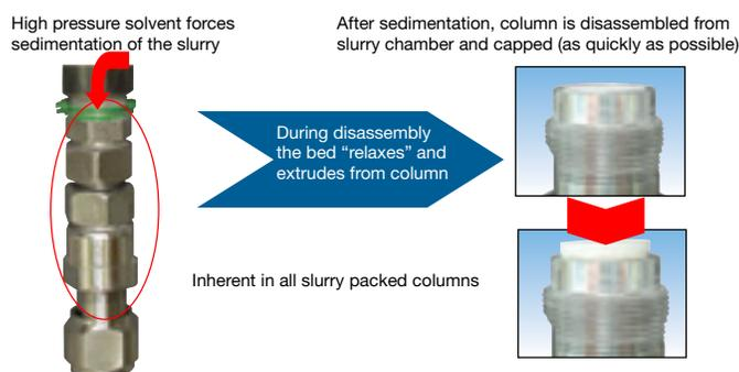
With slurry packed columns, the packing hardware must be disassembled before the end fitting is placed on the column. During this procedure the pressure on the media must be released, the packed bed is disturbed and the media begins to extrude from the column creating non-uniform density.
