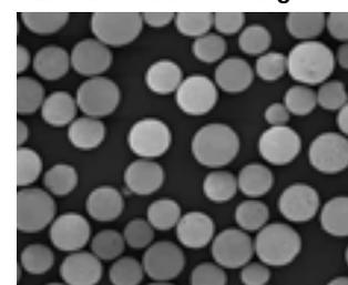
Lux media is mechanically stronger allowing higher packing pressures than previous chiral media.
